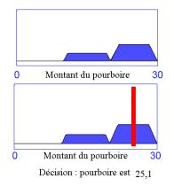
Figure 1.11: Defuzzification with the method of the mean of maxima (MeOM)
