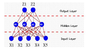
Figure 3.10: Example of a feedforward neural network
