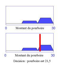
Figure 1.12: Defuzzification with the method of center of gravity (COG)
